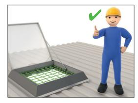
**Prevent falling** through by using safety mesh
